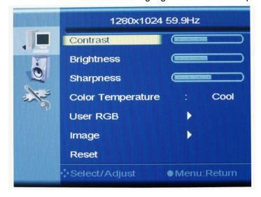
b. Press " " or " " to increase or decrease the contrast of the display. Then press "1" to confirm the adjustment and back to OSD main menu.
